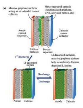
The large surface areas of the SMCs' electrodes enable rapid shuttling of large numbers of ions between electrodes, resulting in a fast recharge time. Image copyright: Jang, et al. ©2011 American Chemical Society
