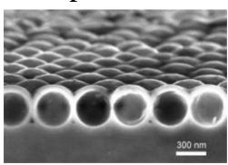
This scanning electron microscope image shows a cross section of a layer of hollow nanoshells made of photovoltaic silicon. The thin spherical structure improves light absorption by trapping the light inside the material, creating what are known as optical whispering galleries. Credit: Yan Yao
