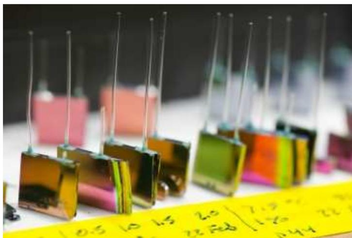
A variety of silicon chip micro-reactors developed by the MIT team. Each of these contains photonic crystals on both flat faces, with external tubes for injecting fuel and air and ejecting waste products. Inside the chip, the fuel and air react to heat up the photonic crystals. In use, these reactors would have a photovoltaic cell mounted against each face, with a tiny gap between, to convert the emitted wavelengths of light to electricity.
